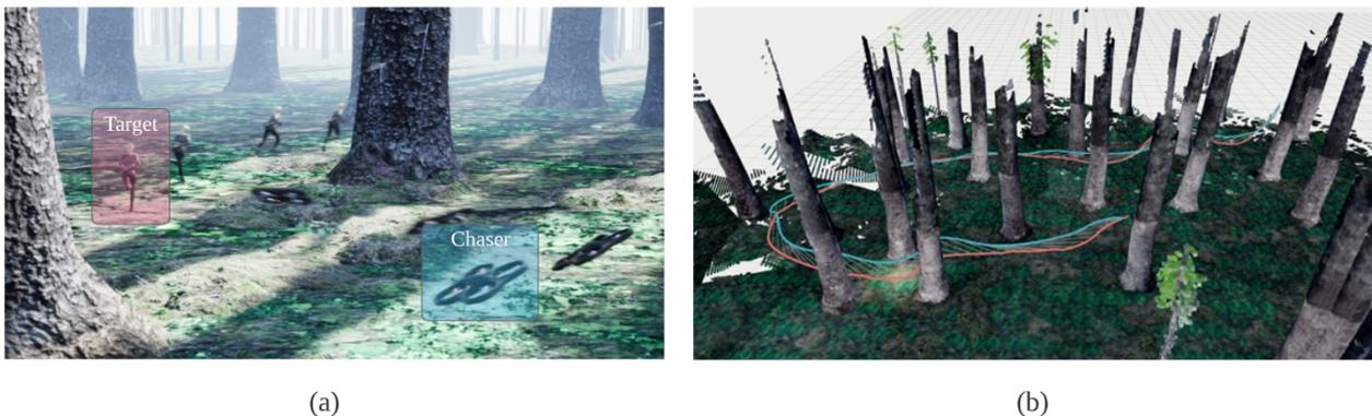
**Fig. 1 (a)** Autonomous chasing for a dynamic actor with a drone in a dense forest. The actor moves at 2 m/s speed, whose trajectory is not known a priori to the chaser. **(b)** The translational histories of the drone (sky-blue) and the target (pink). By reducing collision or target-occlusion, the drone operates in a receding horizon manner using the proposed pipeline.
