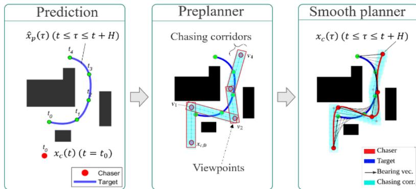
Fig. 4. The proposed chasing pipeline.
