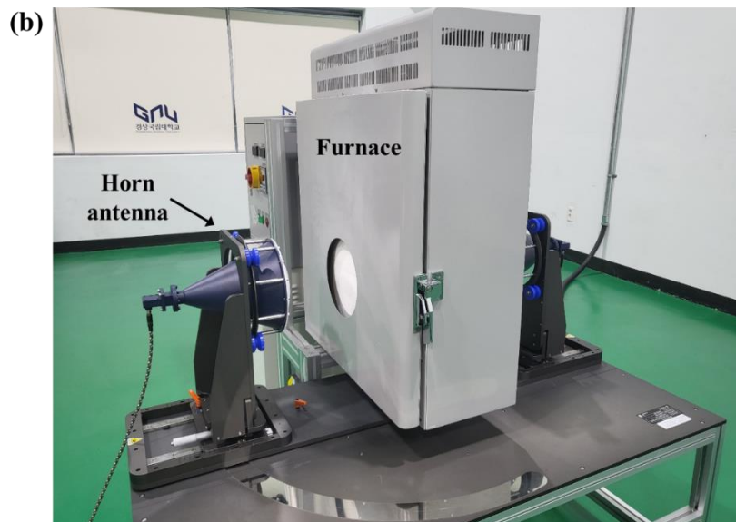
Figure 10. (a) Schematic and (b) equipment of the free-space measurement system with ultra-high temperature furnace
