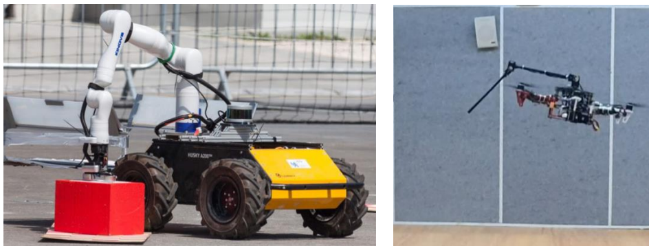
Figure 1 (a) A ground-based mobile robot and (b) an aerial manipulator
