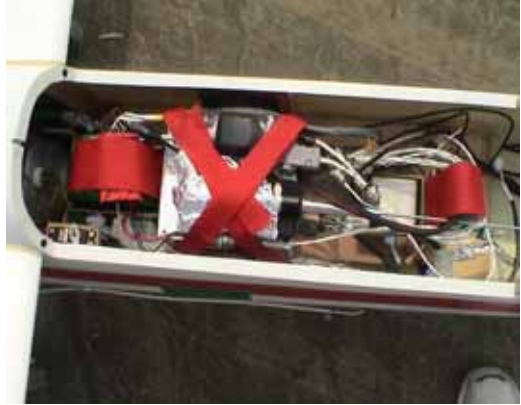
Fig. 22 FCC Equipped on the Fuselage of the CNUAV-
