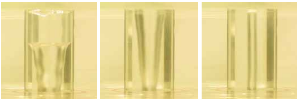
Fig. 11 The transient inner flow of the backhole region
