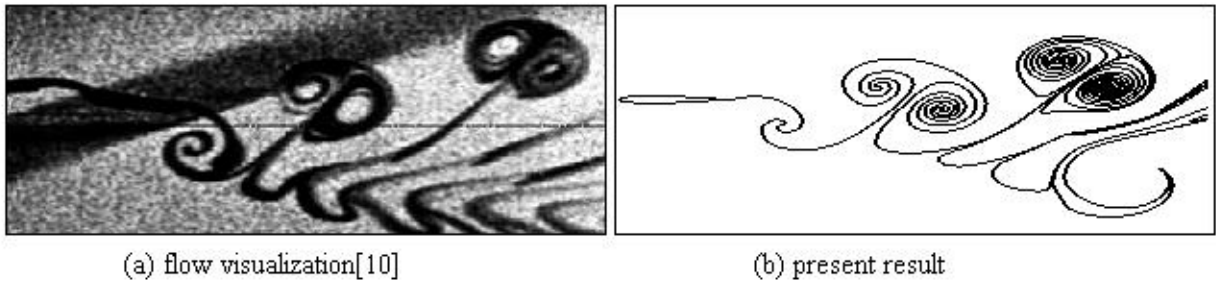
Fig. 8 Comparison of wake pattern behind an plunging airfoil for k=10, k_0=0.2
