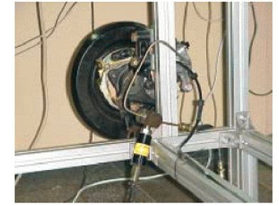
3. Integration module of ECU( ), Coupling of brake equipment with pressure sensor( )
