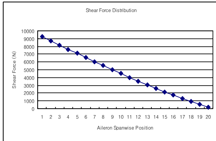
Fig. 14 Shear force diagram of aileron
